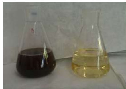
Figure 4. Sample of WW from the steam chamber before the treatment and after the second step of the treatment by ferrate (VI).
