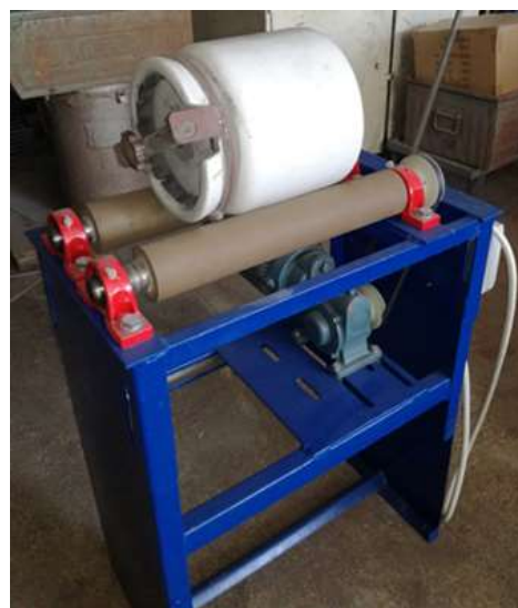
Figure 1. Appearance of the rotary ball mill, in which the reactions take place.
