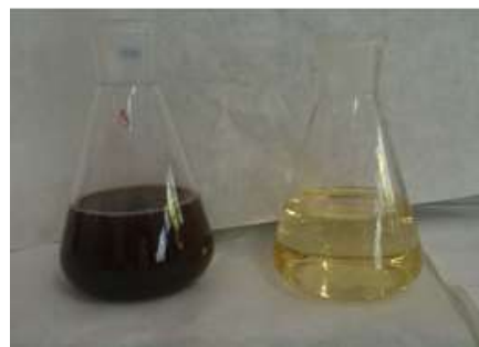
Figure 4. Sample of WW from the steam chamber before the treatment and after the second step of the treatment by ferrate (VI).
